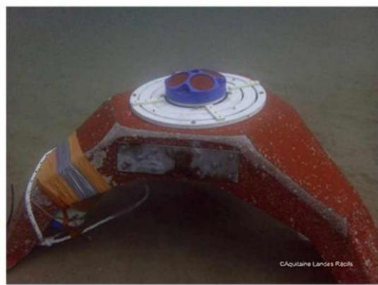
Figure 40 ADCP immergé sur la concession de Capbreton (2017) Source: ALR
